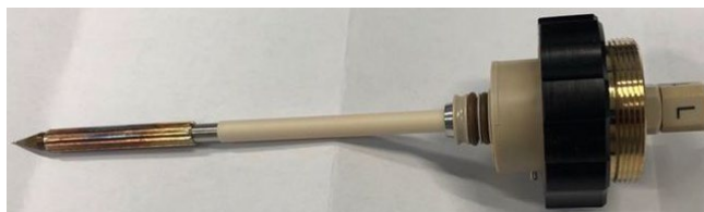
Figure 133: Low flow needle insert "L" (P/N OPTON-30697 Kit). Adjust the needle position closest to the ion transfer tube horizontally (to 1) and vertically (to L).
