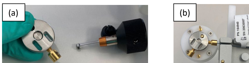
Figure 113: Low dispersion Y-piece with Viper Blind Plug Installed (and alignment retaining plug removed) (a) Low dispersion Y-piece attached to the column inlet and mounted on DBO Liquid Junction Holder (b)
