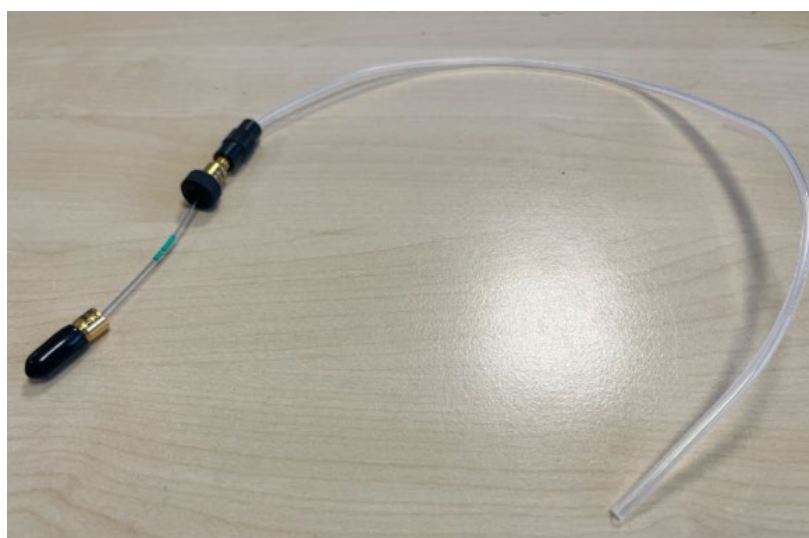
Figure 87: Waste line capillary which permits flow meter purging on the separation pump (P/N 6079.2425). The capillary is shipped with 2.5 meters of FEP (Fluorinated Ethylene Propylene) waste tubing which should be cut to the appropriate length prior to first use
