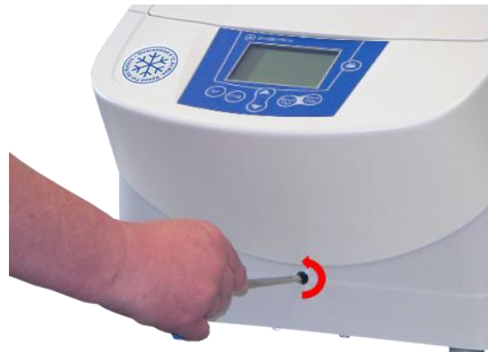
Fig. 15: Manual release of the lid lock
