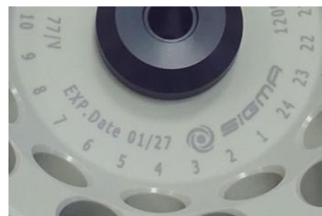
Fig. 5: Different service life – engraving on the bucket/rotor
