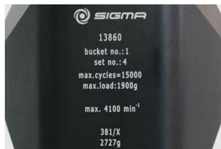
Fig. 5: Different service life – engraving on the bucket/rotor
