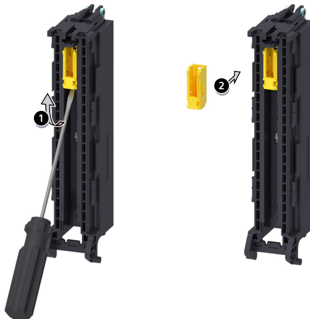
Figure 15-10 Removing the electronic coding element from the front connector and inserting it into a new front connector
