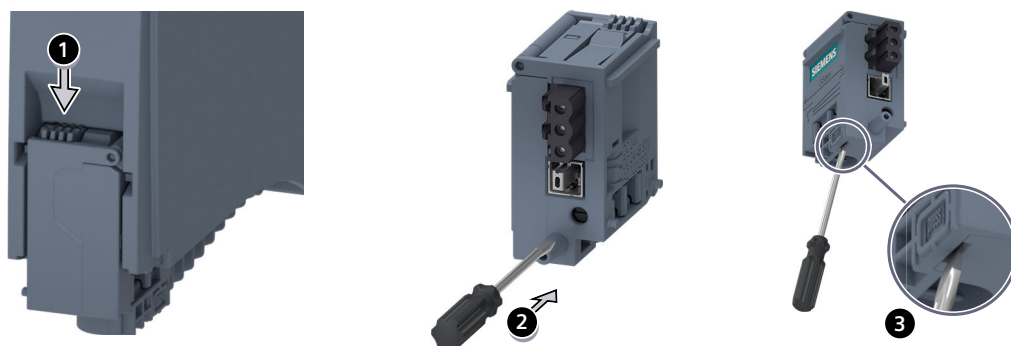
Figure 8-6 Connecting the supply voltage to a system power supply/load current supply (1)
