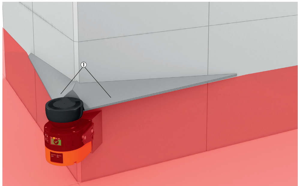
Figure 17: Mounting with deflector plates (example)
