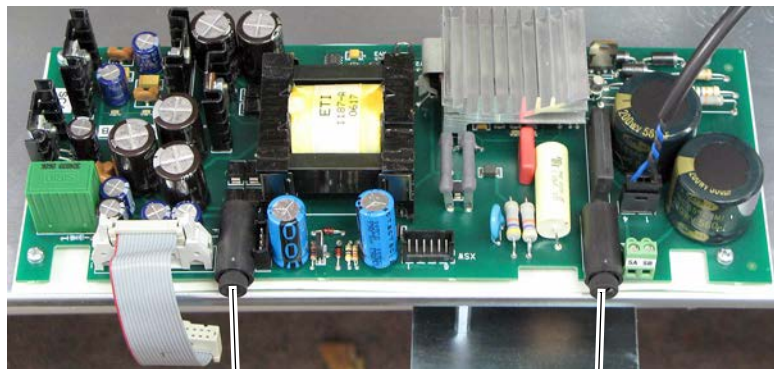
Figure 81 - Frame C Switching Power Supply Circuit Board Fuse Location
