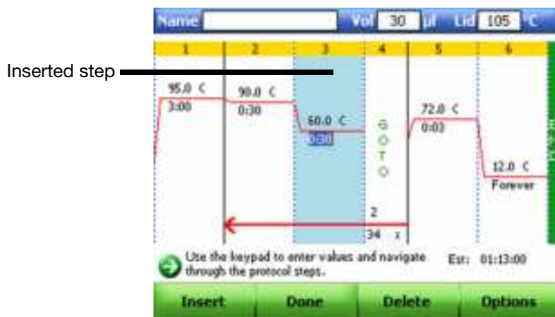
Figure 35. A temperature step inserted inside a GOTO repeat.
