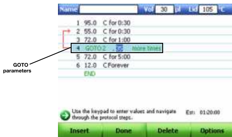
Figure 49. Protocol with GOTO parameters shown in textual view.
