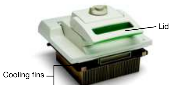
Figure 4. The lid and cooling fins of a 96-well reaction module.
