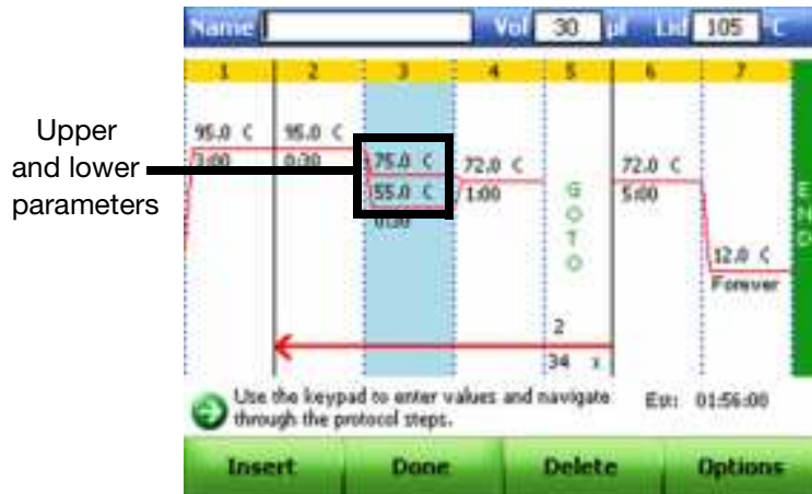
Figure 40. The gradient range changed from 55 to 75°C.
