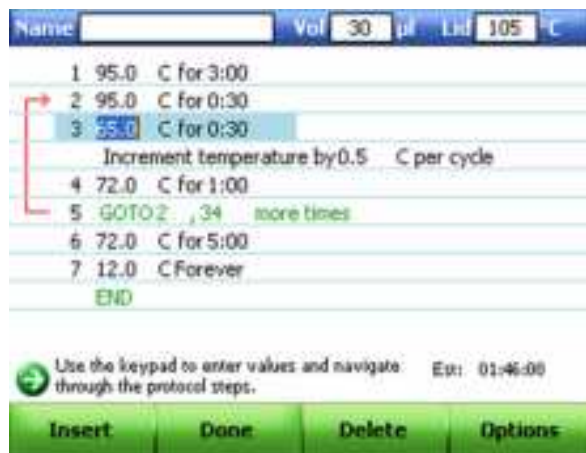
Figure 42. An example of a ramp changed in step 3 of the protocol.
