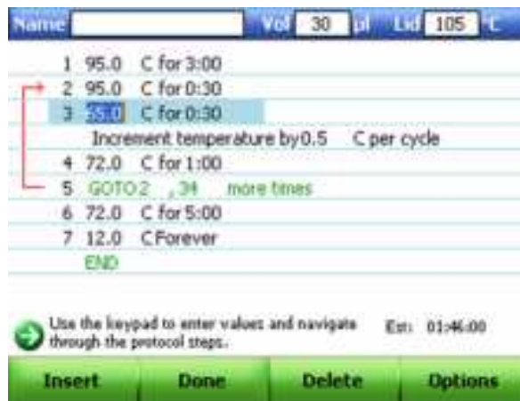
Figure 41. A temperature increment added in step 3 of the protocol.
