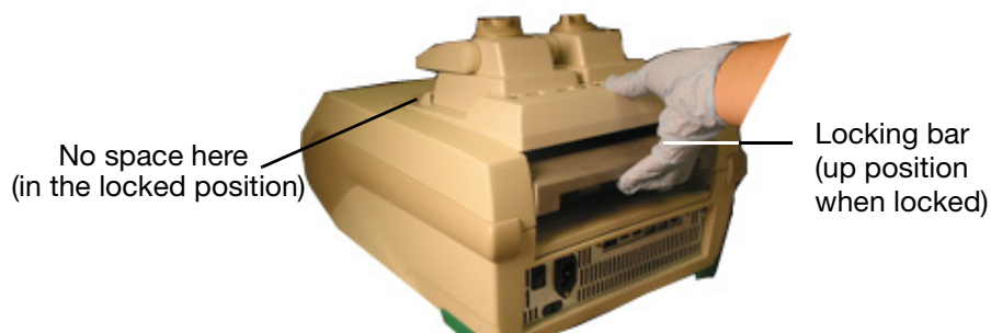
Figure 7. Locking the reaction module in place.
