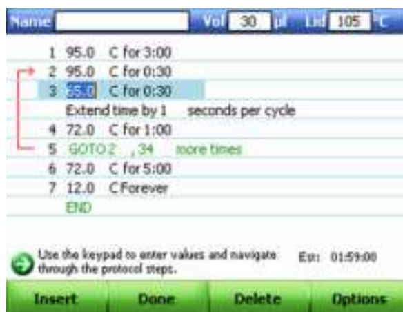
Figure 43. An extend time is added to step 3 of the protocol.
