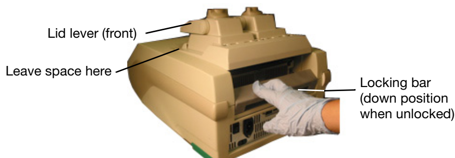
Figure 6. Inserting the reaction module into the bay.
