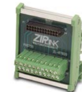
ZL-RTB20 20-pin feed-through connector module
