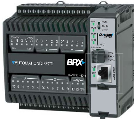
BX 18E Micro PLC Unit (MPU) with Built-in Analog and Ethernet Port
